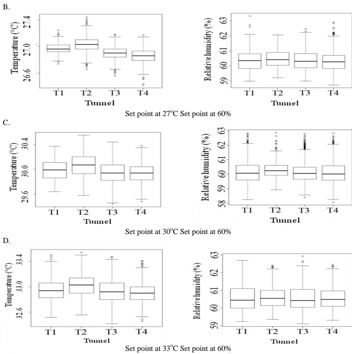
Figure 6. Boxplots for the temperatures of 24 (a), 27 (b), 30 (c) and 33 °C (d) and relative humidity at 60% for each wind tunnel (T1, T2, T3 and T4)
