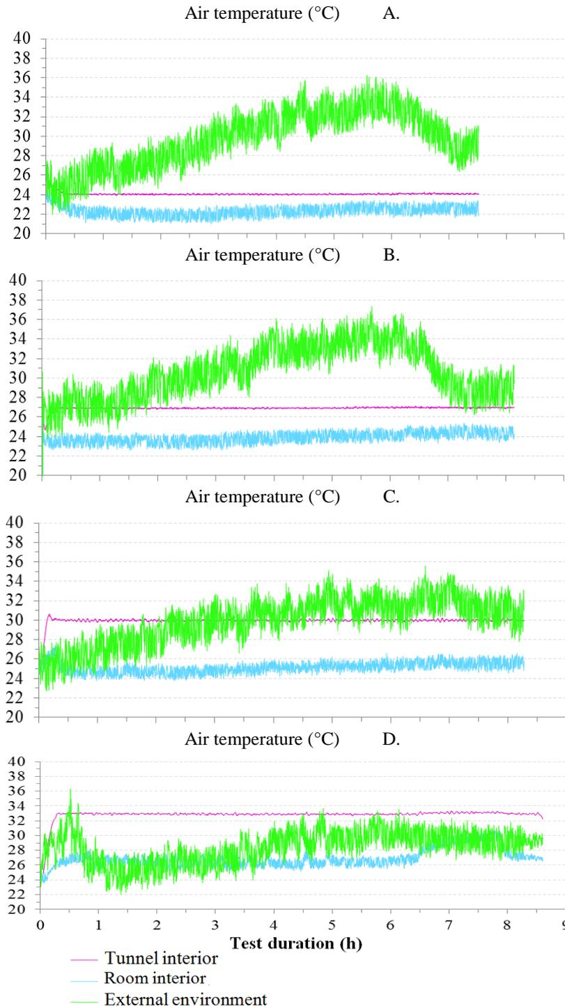
Figure 7. Behavior of the air temperature inside the wind tunnel, inside the room and in the external environment for the set points at 24 (a), 27 (b), 30 (c) and 33 °C (d)
